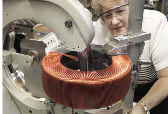
Coil Winding for VT, Test Set, and Voltage Regulator Applications
